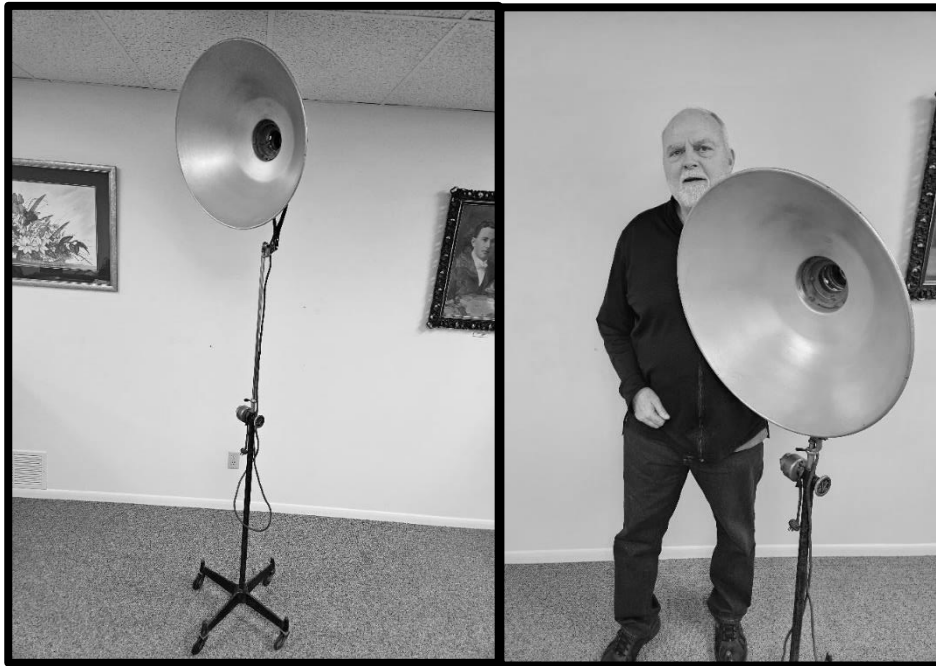
One of thirty floodlights, fully extended to 8' compared to itself when fully retracted at 5'.
